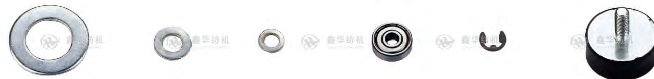
XH-V1310 Name: Gasket No: 0128002 Notes: Φ21 XH-V1311 Name: Flat gasket No: 0123001 Notes: Φ8.4 XH-V1312 Name: Flat gasket No: 0122001 Notes: Φ6.4 XH-V1313 Name: Bearing No: 0130101 Notes: 626 XH-V1314 Name: Circlip No: 0171001 Notes: Φ6 XH-V1315 Name: Rubber stick No: 0463008 Notes: M10*50
